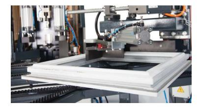
Single Line 1 Four Head Welding and CNC Corner Cleaning Machine
